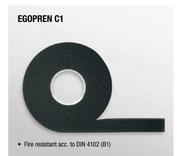
EGOPREN C1 is a precompressed, impregnated polyurethane soft foam sealant strip that is self-adhesive on one side, meets the requirements of DIN 18542-BG1 and is fire resistant according to DIN 4102 (general building inspection test certificate available). The product is supplied in rolls. After positioning the material expands gradually according to temperature and adapts to the width of the joint and to uneven surfaces.
