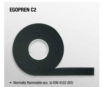
EGOPREN C2 is a precompressed, impregnated polyurethane soft foam sealant strip that is self-adhesive on one side, meets the requirements of DIN 18542 BG2 and is normally flammable (B2) acc. to DIN 4102 (general building inspection test certificate available). The product is supplied in rolls. After positioning the material expands gradually according to temperature and adapts to the width of the joint and to uneven surfaces.
